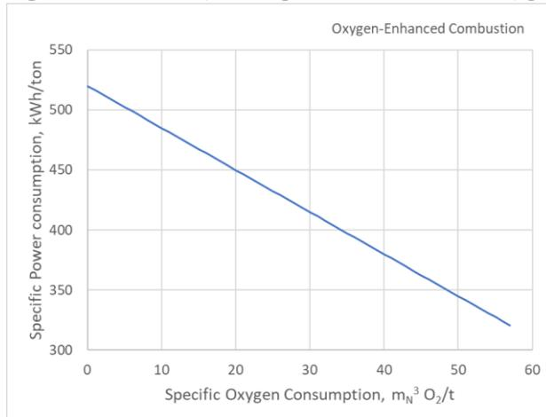
Sources: CO<sub>2</sub> abatement in the iron and steel industry; Anne Carpenter, 2012; Oxyfuel combustion in the steel industry: energy efficiency and decrease of CO<sub>2</sub> emissions; Joachim von Schéele, The Linde Group Germany
