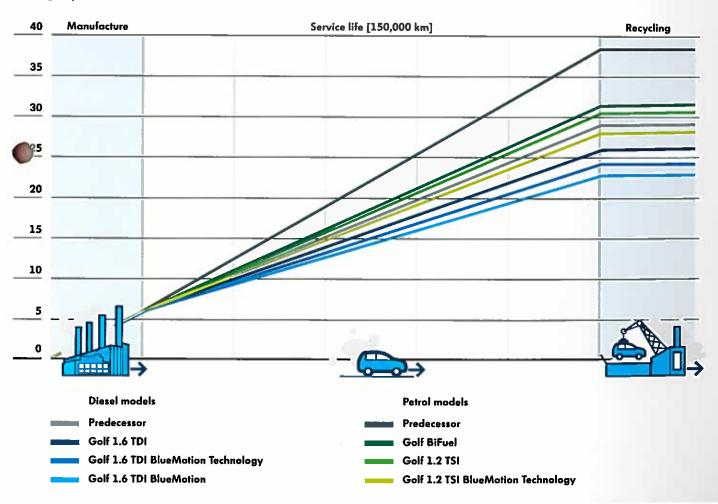
For an assumed lifetime mileage of 150,000 kilometres our calculations for the diesel models indicate life-cycle emissions (measured in  $CO_2$  equivalents) of 26.2 metric tons (1.6 TDI), 24.3 metric tons (BlueMotion Technology) and 23.1 metric tons (BlueMotion). This means that the 1.6 TDI shows a 10% improvement over its predecessor, while the BlueMotion Technology model records an improvement of 17% and the Golf BlueMotion 21%.
