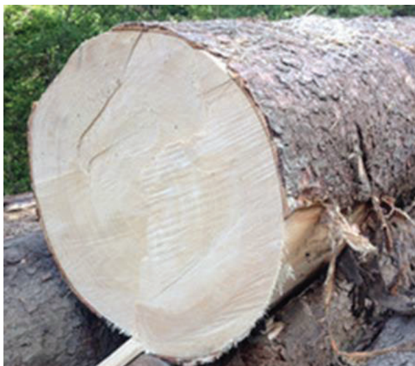
Figure 2 Example of a good quality spruce log which can be used for sawn goods. Picture Sylvain Ougier CNPF
