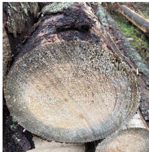
Figure 3 Spruce log with discoloration made by a fungus. Due to visual defects this log is not suitable for sawn goods or pulp. Picture by Patrick Lindenbjär.
