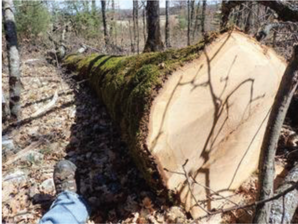
Figure 4 Example of a good quality oak log: straight and without defects. Picture Mael Grauer CNPF.
