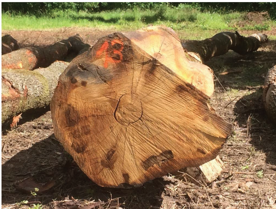
Figure 3 This large diameter oak log is rotten and curved. The rotten parts cannot be used for sawn goods and oak is not a suitable raw material for pulp. This rot is only detectable after felling. The curve of the stem makes it difficult to use it for sawn goods. Picture Luc Bouvarel.
